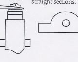
Anvil fullers may be used for drawing stock with the flat face in the hammer. You can also use a handled top fuller with the bottom fuller or with the flat face in the anvil.
