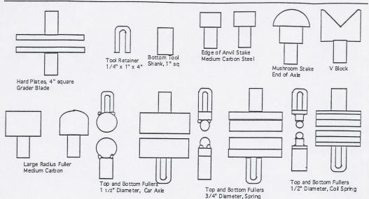
These are some of the tools I use most in the hammer and the anvil of the TH. The tool retainer must be welded on top of the top tools. Many types of tool steel do not weld readily. 7018 rods are best used when welding medium or high carbon or other tool steel. Many times you can make a successful weld by preheating (and post heating) the stock to at least 400° F before stick welding. Sometimes MIG welding is OK if you get enough penetration-requires a bigger MIG than the 110V jobs.
