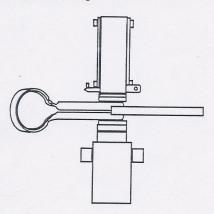
The spring fuller is great when you are doing operations with several different tools in one heat. Sometimes if the spring closes it may be difficult to get the work between the fullers. Put the stock in the spring loop and pull out to the working area or put the thin dimension of the work between the fullers and twist to open.
