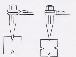
for the full length and turn over to the opposite side. Keep all cuts centered and keep the cutter vertical.
