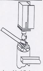
Get a smooth finish by using a flatter on flat or tapered stock. The hammer and anvil hard plates may be used as flatter on
